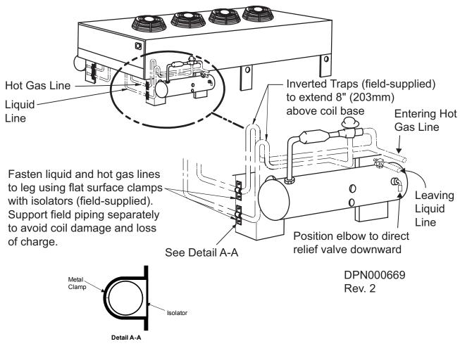
Figure 23 Lee-Temp head pressure control condenser piping
